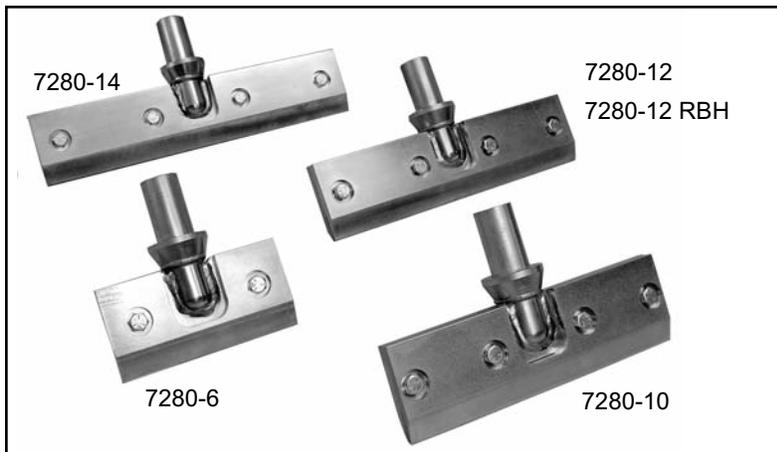
**CUTTING HEADS:** Unique swivel cutting head assemblies. Swivel head allows blade to stay in contact with the floor. Razor Blade Head (RBH) is designed to hold Razor Blade.
